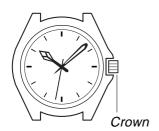
Pull the crown out. Set the hands by turning the crown in either direction. Push the crown in on a time signal.
