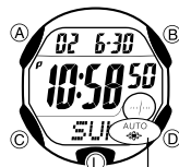
Auto light switch on indicator
