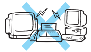
Next to a household appliance or office equipment (TV, speaker, fax, PC, etc.)
