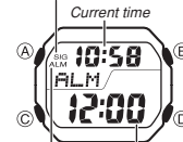
Alarm on indicator
