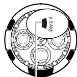
Power saving indicator
