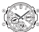
Auto light switch on indicator
